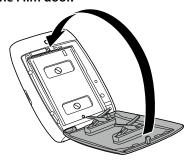
4 Remove the black film cover that is automatically ejected from the printer.
