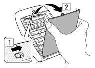
Insert an INSTAX MINI instant film pack by aligning the yellow marks on the film pack and the printer body.
